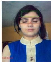
Fig. 5 Closed Eye Detection
